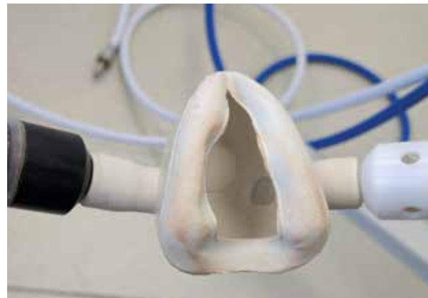
Figure 2 (Left) MDM with cleaning damage
