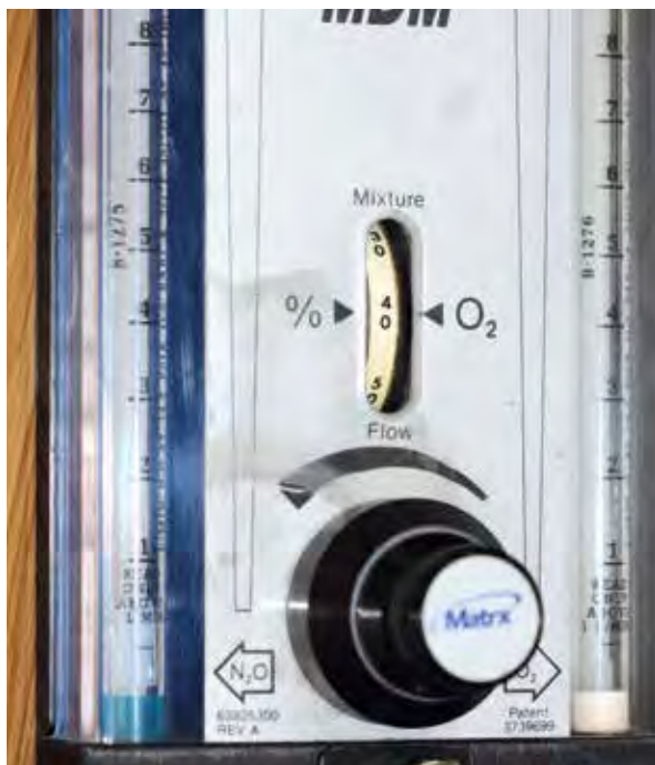
Figure 2 (Left) MDM with cleaning damage
