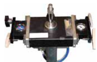
Fig 4 Old Cyprane 4-cylinder stand yoke assembly
