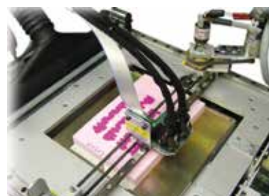
FIGURE 1D 3-D printing of brackets in wax polymer
